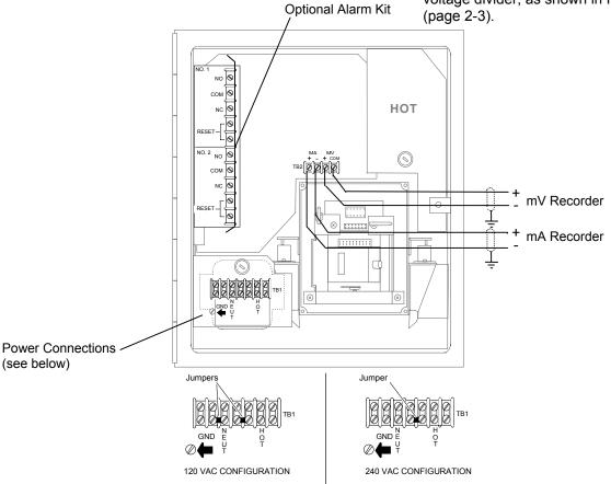
Figure 2-1. Electrical Connections
